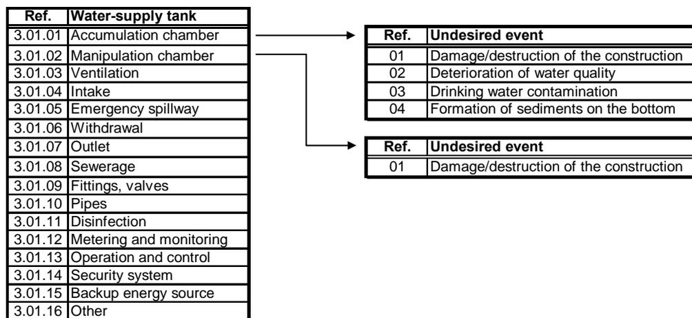
**Figure 1.4** Example of defined undesired events for some elements of water-supply tank
